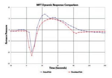
**Benefits:** Avoid unnecessary boiler stiffening for conversion of forced draft to balanced draft operation (costing in excess of several million U.S. dollars). Develop MFT control logic which prevents implosion damage to a boiler.
