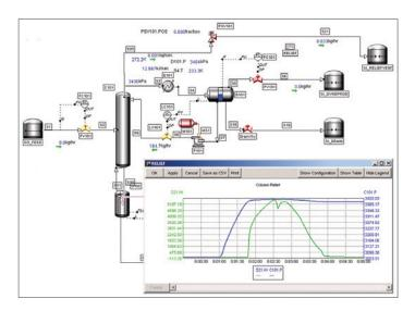
For fractionation towers with wide boiling ranges: flare load reductions (up to 50%) are possible as dynamic simulation accounts for the limited inventory of light components and the sensible heat required to boil off the heavier components. Dynamic simulation also provides a realistic calculation of the reboiler pinch at elevated pressures using the time-dependent feed
